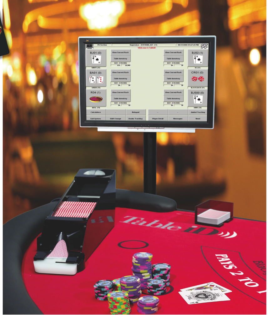
Figure 2 The Table iD system collects information from RFID chips and card readers to provide a snapshot of each player's gambling activity.
