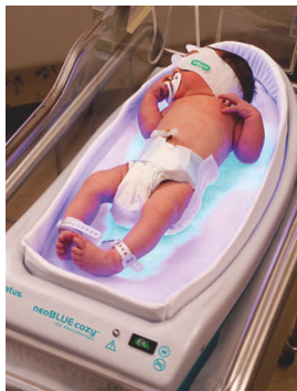
Figure 2 Blue LEDs, like those in this bassinet system from Natus Medical, target the most effective blue-light spectrum of 458 to 462 nm for the treatment of hyperbilirubinemia in infants.
